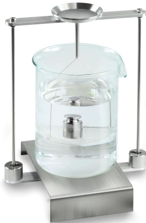
Figure 2: Weighing in auxiliary liquid
