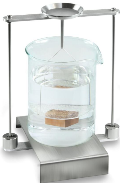
Fig. 4: Weighing in auxiliary liquid
