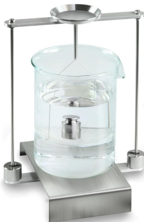
Fig. 2: Weighing in the auxiliary liquid
