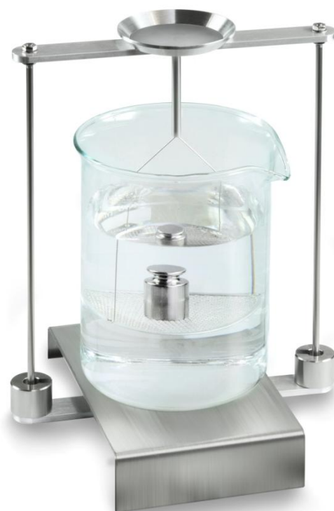
Figure 2: Weighing in auxiliary liquid
