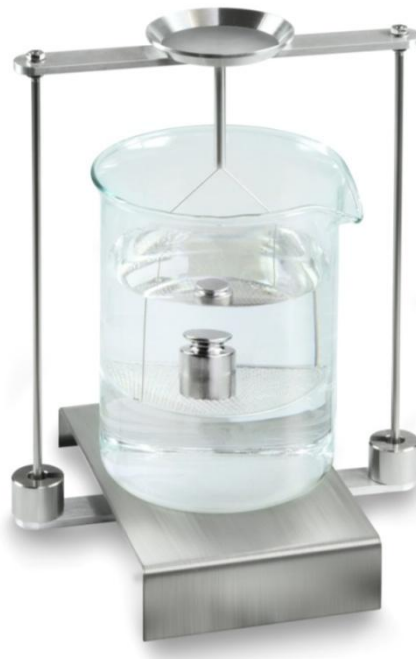
Fig. 2: “Weighing in auxiliary liquid”
