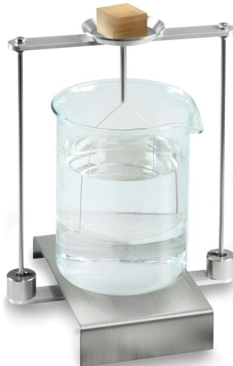
Fig. 3: Weighing in air
