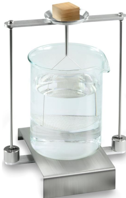
Fig. 3: Weighing in air
