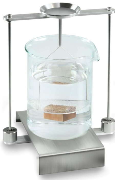
Fig. 4: Weighing in the auxiliary liquid
