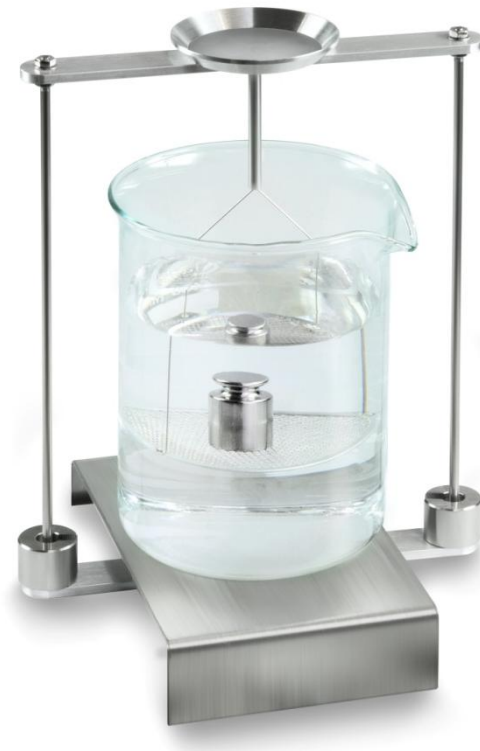
Fig.6: Weighing in test liquid
