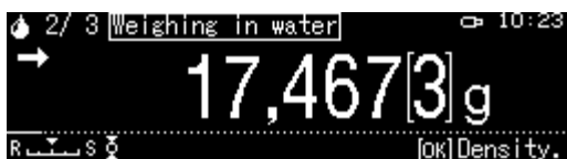
Fig. 2: Weighing in the examined liquid
