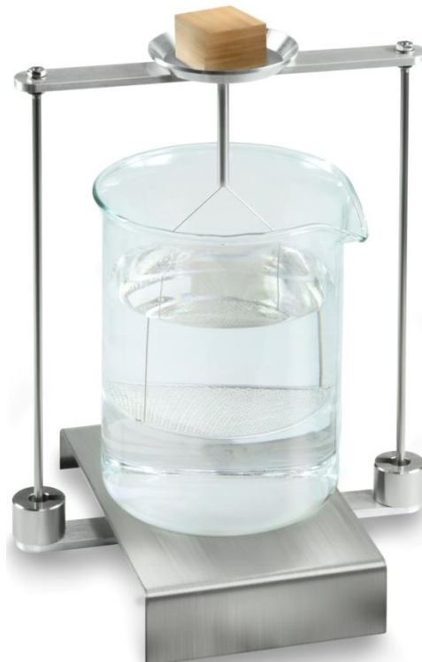
Fig. 3: Weighing in the air
