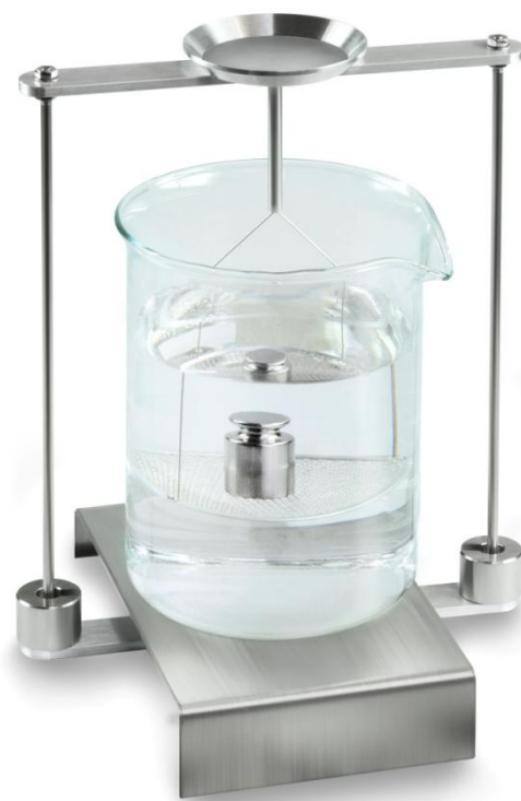
Fig. 2: Weighing in the examined liquid
