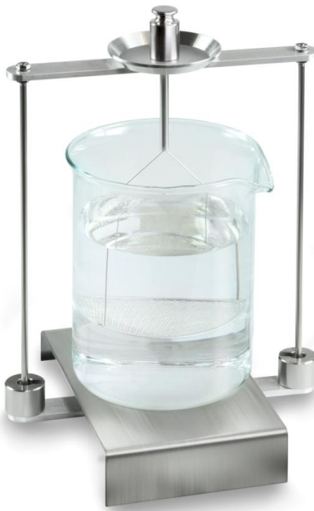
Fig.1: Weighing in air
