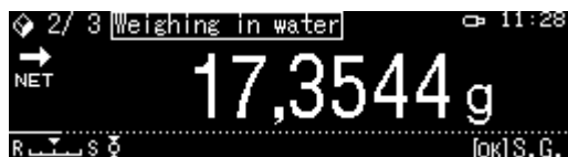
Fig. 2: Weighing in the auxiliary liquid
