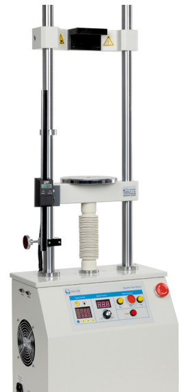
Motorised test stand incl. length measuring device LB
