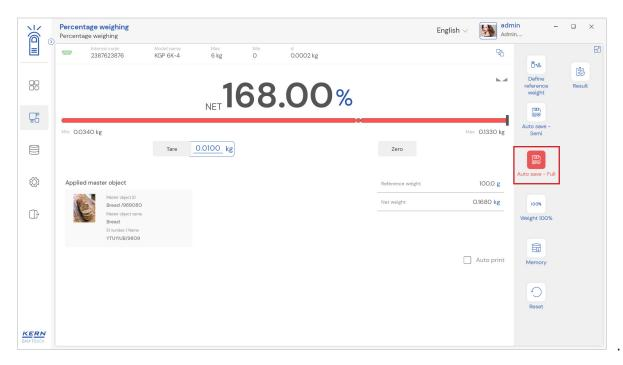
Step 2: Place the object that is required to find the percentage Step 3: Wait until the weight on the scale is stabilized
