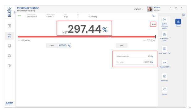
• The net weight along with the reference weight would be displayed in the screen for user's
